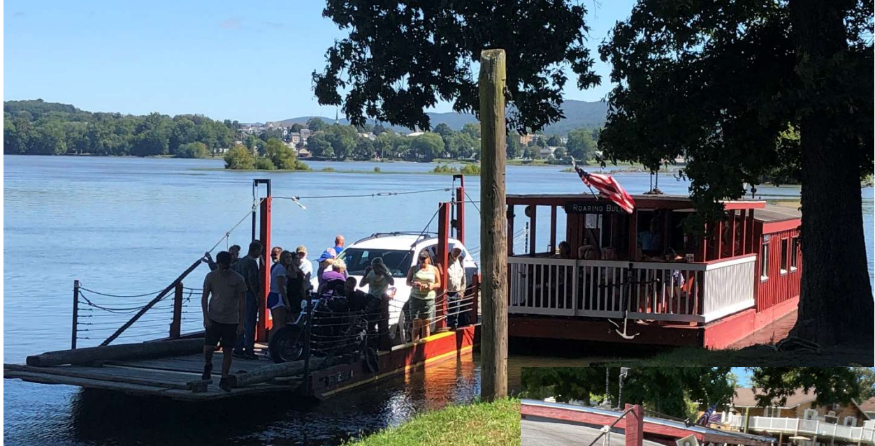
The primitive Millersburg Ferry consists of a flat barge lashed to a paddle wheel tug. It can hold maybe 5 cars or 20 motorcycles.
