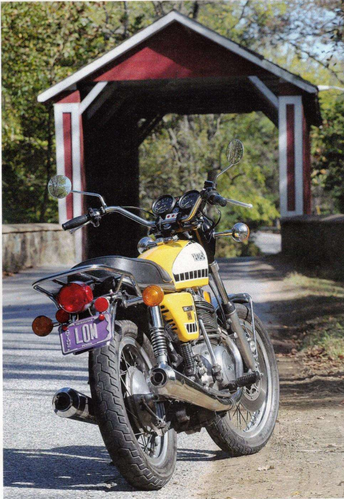
The 743cc air-cooled twin makes 63 horsepower at 7,500rpm.
