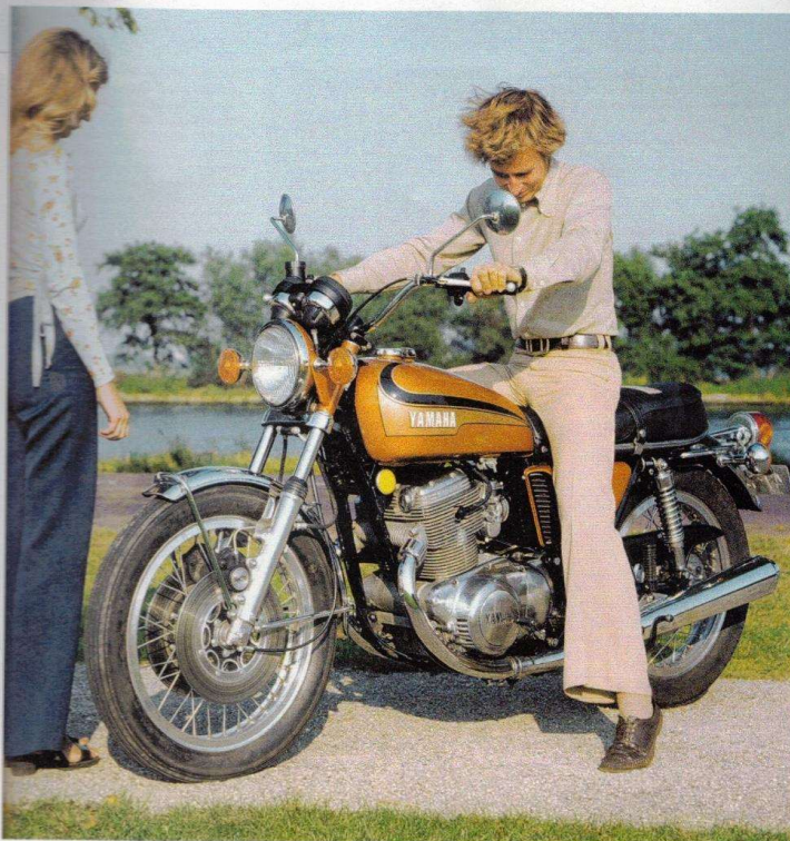
The single-disc front brake's performance is lackluster at best. The fork has a boss for a second disc, but U.S. models only got one. Racer Jarno Saarinen and wife Soeli in a PR photo for the TX750, circa March 1973.
